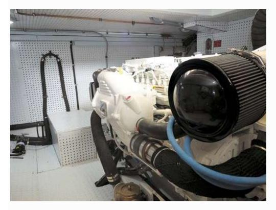
Engine access aboard the Integrity 47XL Grand Sedan was through a hatch in the saloon floor and down an easily accessed ladder. With only a single engine in the beamy and clean enclosure you have acres of space for maintenance. Head height is limited but the non-skid rubber mat means you have a soft floor to move on.
