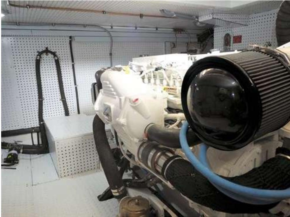
Engine access aboard the Integrity 47XL Grand Sedan was through a hatch in the saloon floor and down an easily accessed ladder. With only a single engine in the beamy and clean enclosure you have acres of space for maintenance. Head height is limited but the non-skid rubber mat means you have a soft floor to move on.
