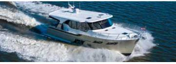
Volvo D11 670 HP. Topspeed 22 knots Semi-displacement hull
